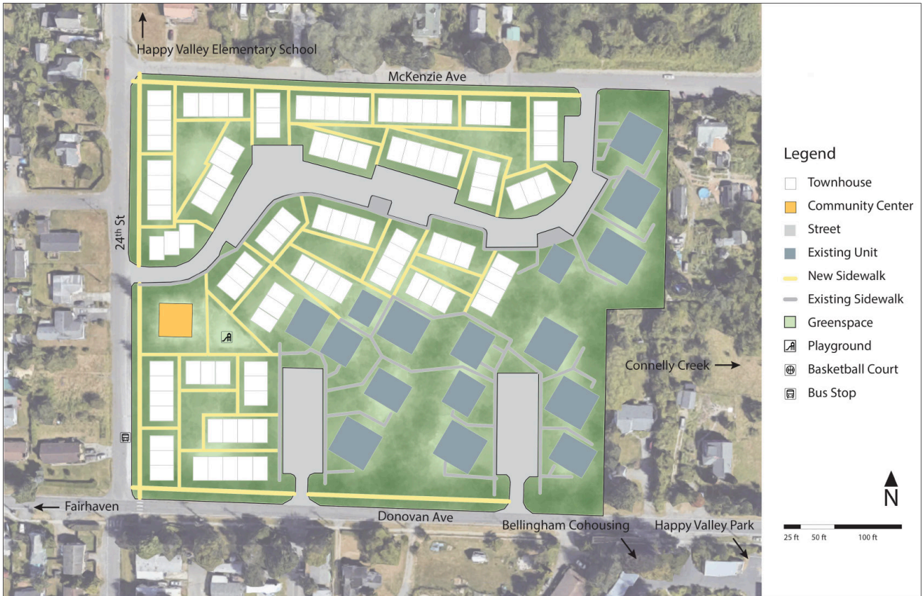
Figure 10. The site plan for Alternative C, which has 161 total units. Source: UW Team.
